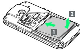
· Slide battery into place as shown.
