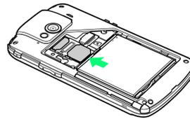
· Slide in USIM Card with IC chip down.
