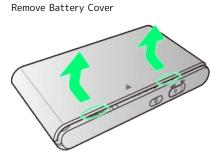
$\cdot$  Press where circled  $\bigcirc$  (beveled surface) to slide as marked  $\bigtriangleup$  on Cover, and lift it up to remove it.
