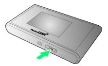
• Push in USIM Card Tray, and check that USIM Card is completely installed.
