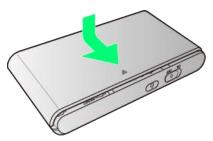
$\cdot$  Check the orientation of Battery Cover, and place it on Wi-Fi router, slide it in the direction shown until it fits in place.
