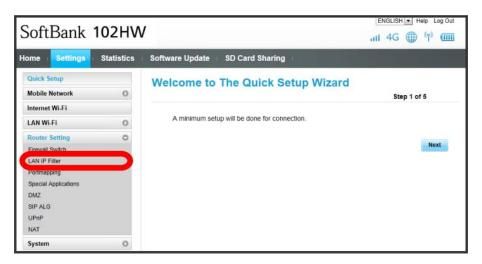
· If a message asking to enable IP address filter appears, enable "IP address filtering" from Firewall Switch and retry.
