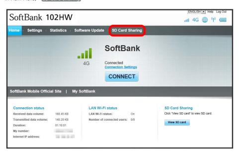
· To share Memory Card data, log in to SoftBank 102HW Utility. Although SD Card Sharing window can be shown without logging in, to change settings, click "Log In" at the right top of the window to log in.
