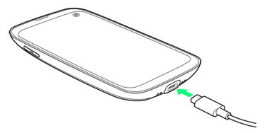
■ Holding plug by connector, insert without bending as shown.
