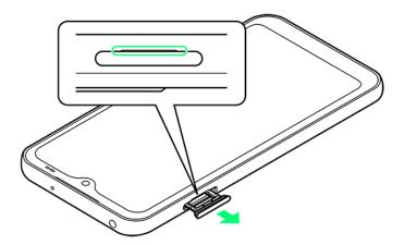
■ After use, insert Slot Cap straight without bending in direction shown, and press firmly where circled ○. Make sure there is no gap between handset and Slot Cap.
