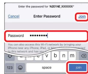
When connection is successful, the WLAN connection counter number on the Status Indicator of the Wi-Fi router increases by one.
