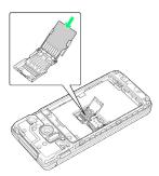
$\cdot$  Check orientation of SD Card, and slide in direction shown to insert in Cover.
