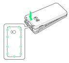
$\cdot$  Fit on handset, press firmly where circled (O) ensuring no gaps.
