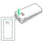
$\cdot$  Fit on handset, press firmly where circled (  $\!\!\!\!\bigcirc$  ) ensuring no gaps.
