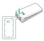
$\cdot$  Fit on handset, press firmly where circled (O) ensuring no gaps.
