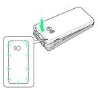
Fit on handset, press firmly where circled (O) ensuring no gaps.
