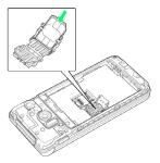
· Check orientation of USIM Card (notch/IC chip), and slide in direction shown to insert in Cover.
