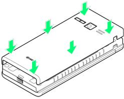
**9**Work way around Back Cover in directions **1** holding down in direction **2** to install completely
