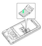
· Note orientation of SIM Card (notch/IC chip (metal) facing down), and place in SIM Card Slot.
