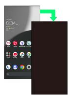
$\cdot$  To activate screen lock manually, Press Power Key when Display is turned on.
