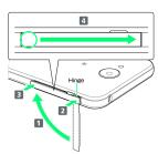
Lift Card Slot Cap in direction 1, reinsert hinge (2), fit Card Slot Cap so that there is no gap between it and handset, and then push along in direction shown (3). To close, push firmly by sliding with finger from circled area (O) toward hinge (4).
