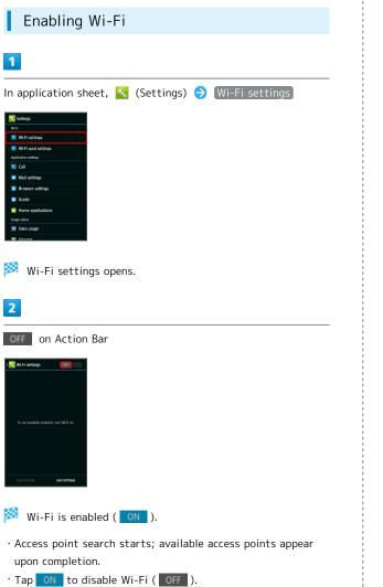
Connecting Selected Access Points Enable handset Wi-Fi first. 1 In application sheet, 🔧 (Settings) 🔿 [Wi-Fi settings] 🏁 Wi-Fi settings opens. 2 Tap access point 3 Enter password  $\Rightarrow$  Connect 🏁 Handset connects to selected access point.  $\cdot$  Password (indicated by WEP, WPA, KEY, etc.) may be found on a label on your Wi-Fi router. For details, contact the vendor of the router. For public wireless LAN services, check the password with your ISP.
